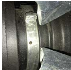
Labyrinth lubrication of shaft oil seal rings
